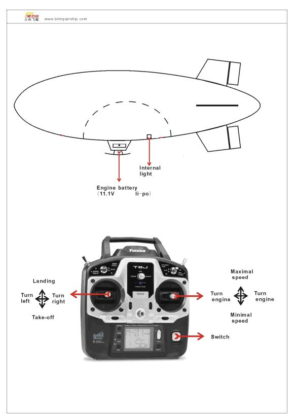
Note: the internal light only can use the 12V battery (3cells Li-Po battery).
